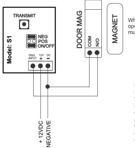
When the magnet opens the contact must close
