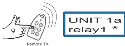
10. To EXIT out of the LEARN/DETETE mode press the MODE button. Then press the Down button till EXIT MODE displays. Then press ENTER.
